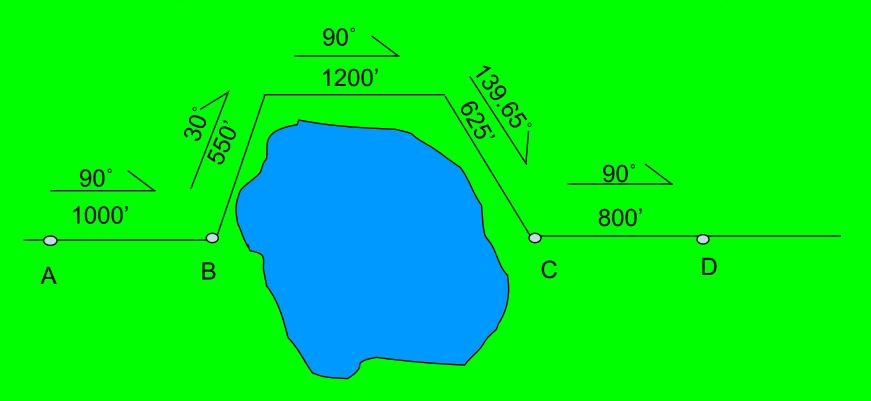
In Laying out a new line, a lake is encountered. Find the straight line distance from point A to Point D. (Note that given angles are compass headings referenced to magnetic north.)
