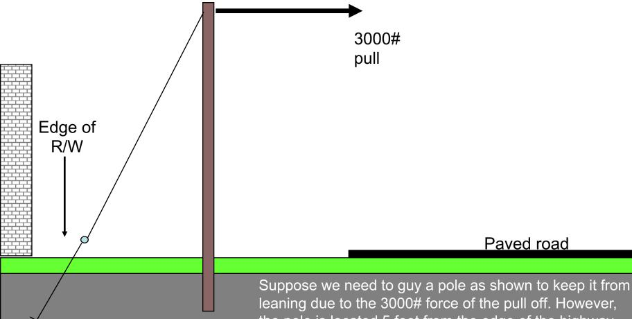
the pole is located 5 feet from the edge of the highway right of way and no easement was obtained to allow guying on the private property behind the pole.
