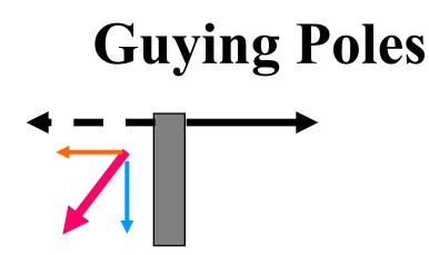
Consider a "free body" diagram of the pole. If the pole is not accelerating in the direction of the pull, then there must be an equal and oppositely directed force balancing the pull on the pole. We will create that force using a down guy and anchor!
