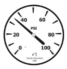
You regularly check the pressure gauge on a large tank. According to the gauge shown, what is the current pressure (in PSI)?
